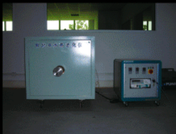
● 觸媒檢測設備-催化器水熱穩定性 測試 Catalyst hydrothermal stability test
